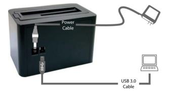
3. Insert 2.5" or 3.5" SATA HDD into the slot.
