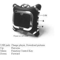
Battery: 3.7V Lithium ion rechargeable battery It will recharge automatically when connect to computer, you can see the battery icon on the top - left of the display.
