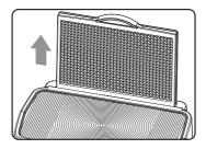
**3** Push the wide angle panel back in, leaving the white reflector card out.
