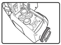
3 Close the battery compartment cover and slide it into place.
