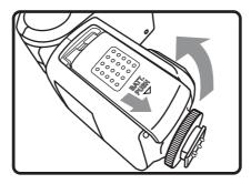
2 Insert four (4) AA batteries (not included). Make sure that the + and – match what is indicated in the compartment.
