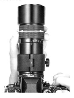
The fully automatic diaphragm of the Micro-Nikkor enables focusing with maximum image brightness throughout the entire focusing range of the lens. As the image is constantly viewed at the maximum aperture setting (i.e., f/4), the depth of field is minimized so that the image snaps in and out of focus rapidly and distinctly.
