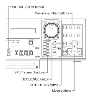
Pressing the OUTPUT A/B button on the front panel switches the multiplexer video output. When OUTPUT A is selected, the button light indicator is off. When OUTPUT B is selected, the button light indicator is on, and camera number buttons, SPLIT screen buttons, and SEQUENCE button are operated for the monitor screen connected to the OUTPUT B connector. Pressing the OUTPUT A/B button again switches the multiplexer output to OUTPUT A.
