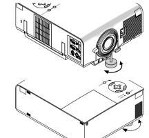
• If the projected image does not appear square to the screen then use keystone correction for proper adjustment.
