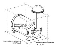
The location of the subwoofer should be based on three considerations: sound coverage, ease of installation, and the ease of running cable to the installation location. The large 10" woofer cone will provide impressive bass performance for a large area when properly placed.
