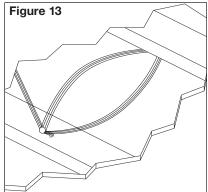
The loudspeaker wire is looped and hung on two nails attached to the joists securing it for future use. Make sure the location is noted on house plans.
