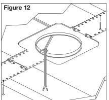
The optional hole saving brackets are installed and the loudspeaker wire is attached to the bracket.
