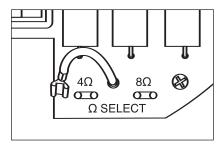
Figure 15 Setting the Impedance jumper.
