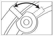
Figure 17 Tightening the mounting "dogs"
