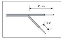
Figure 16 Wire Stripping Details.
