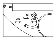
Figure 21 Setting the bass jumper.
