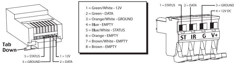
Figure 4 This color code is based on the industry standard T568A coding for the RJ45 connector. When connecting the TS120 to Niles MultiZone Keypads with an IR connection observe this pin configuration
