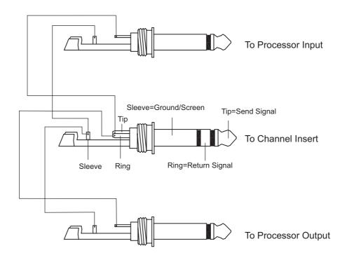
$\rm Y\,\textsc{-}Stereo$  lead for insert Connection (To be used when the processor does not employ a single jack connection for the In/Out Connections)
