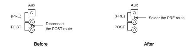
Modification on mono and stereo channels
