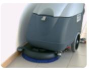
The offset brush deck with side wheel permits efficient close-up cleaning without damaging walls and furniture
