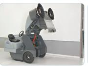
The SR 1900 incorporates superb high-dump capability up to 152 cm from ground level.
