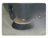
The exclusive DustGuard™ system effectively controls airborne dust by providing a fine mist of moisture to the front and side brushes.
