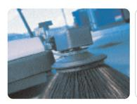
Side brush is easily adjusted and pulls debris away from walls, kerbs, pallets and is easily raised when not needed
