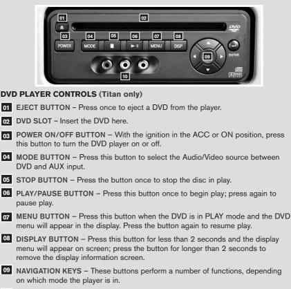
10 INPUT JACKS – These are used to plug additional compatible devices into the DVD system. They are color-coded (yellow – video input; white – left channel audio input; red – right channel audio input).
