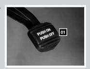
To release, firmly press the foot brake 02, then press the parking brake pedal 01 and the parking brake will release.
