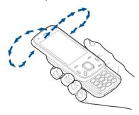
Rotate the device around all axes in a continuous movement until the calibration indicator the changes its colour to green . If the indicator is yellow, the accuracy of the compass is low. If the indicator is red, the compass is not calibrated.
