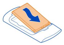
7 Direct the top locking catches toward their slots, and press down until the cover locks into place.
