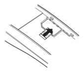
Place the battery on the back of the phone. Slide the battery up the body of the phone until it locks into place.
