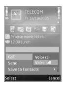
The secondary camera on the front is used by default for video calls. Starting a video call may take a while. Waiting for video image is shown. If the call is not successful (for example, video calls are not supported by the network, or the receiving device is not compatible), you are asked if you want to try a normal call or send a text or multimedia message instead.
