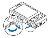
Insert a compatible memory card in the slot. Make sure that the contact area on the card is facing up and towards the slot.
