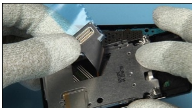
44. Carefully flip the flex foil as shown. Do not fold it!
