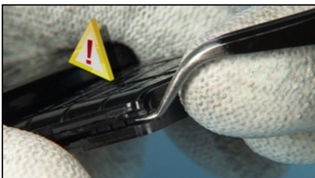
19. Carefully shift the tip of the tweezers outside.
