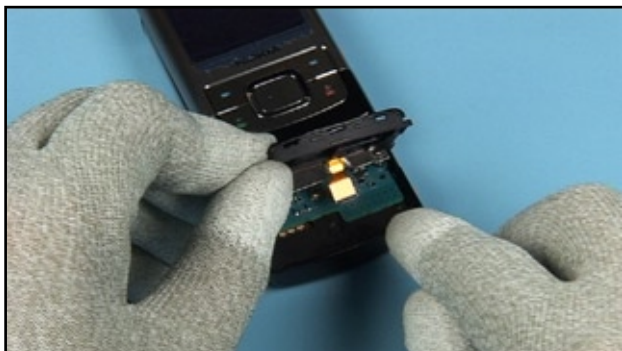
49. Bring the BOTTOM KEYMAT SUPPORT into position as shown. Close the flex foil connector.
