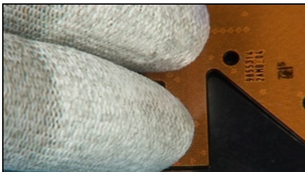
25. Smooth down the TOP FLEX ASSEMBLY evenly.
