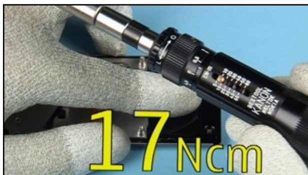
36. Set the correct torque.
