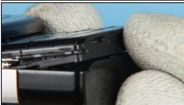
15. Lift up the BOTTOM KEYMAT SUPPORT.
