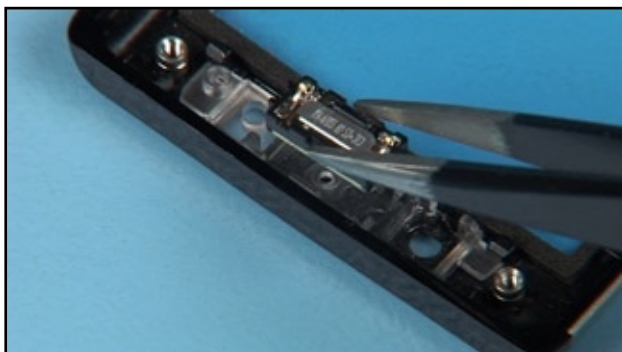
17. Insert the EARPIECE into its compartment.
