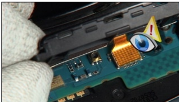
50. Check the correct positioning of the connector.
