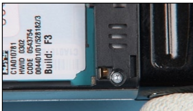
22. The removal of the KEYMAT is also possible without removing the bottom screws.
