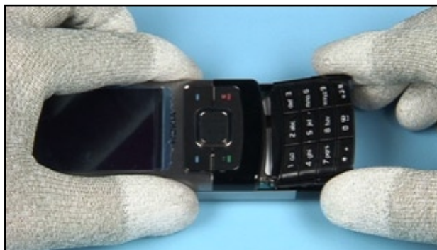
26. Now the BOTTOM KEYMAT can be removed.
