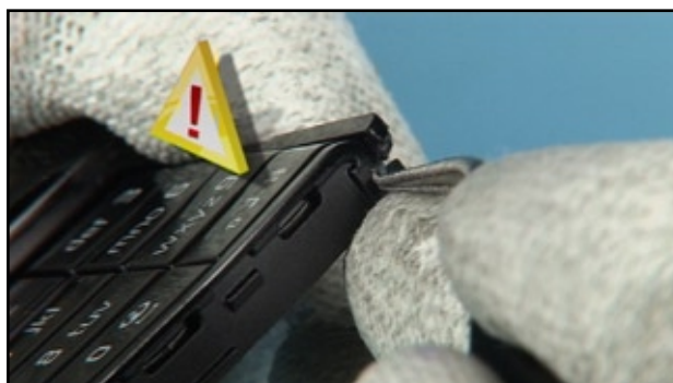
20. Repeat this procedure at the other side of the BOTTOM KEYMAT.
