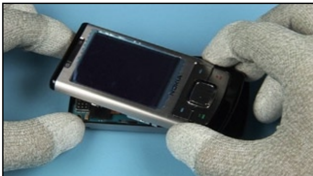
47. Place the upper part over the D-COVER. Do not click it into its place yet.
