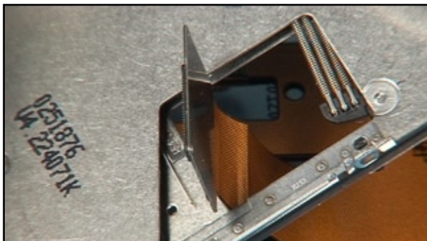
33....to reach the maximum recess. Slot through the flex foil.
