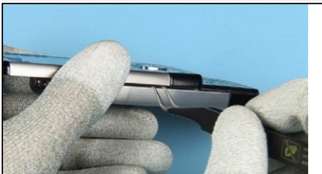
7. Shift open the slider. Carefully insert the tips of the angled tweezers into the recess as shown.
