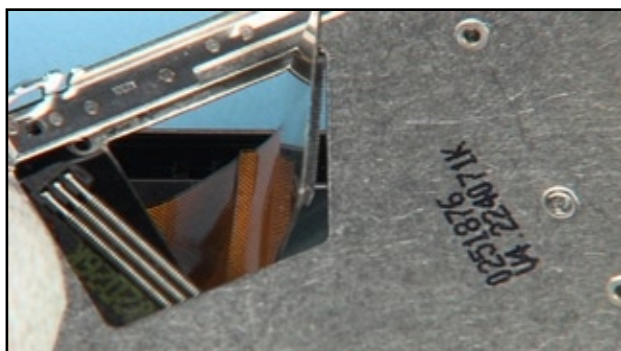
38. Shift the slider into position shown to reach the maximum recess. Slot the connector through the slider.
