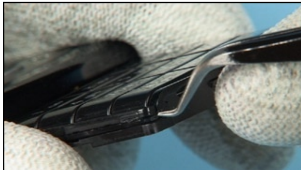
18. Insert the angled tweezers into the recess as shown.
