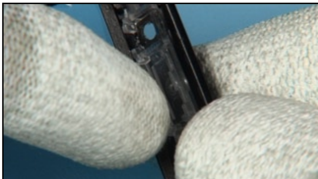
47. Bend the top part of the cover. Twist out the glued in EARPIECE HOUSING ASSEMBLY.
