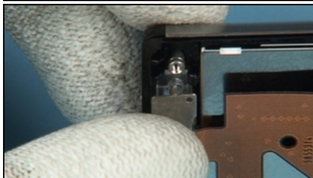
24. Mind the guiding pin of the TOP FLEX ASSEMBLY.
