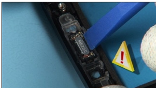
18. Push it down carefully. Never push down the metal part, otherwise the EARPIECE could be destroyed.
