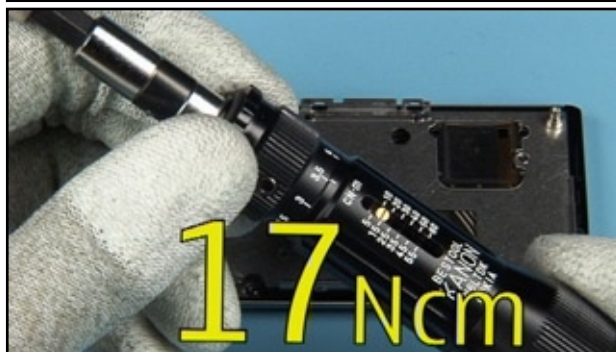
40. Check the torque of the tool.
