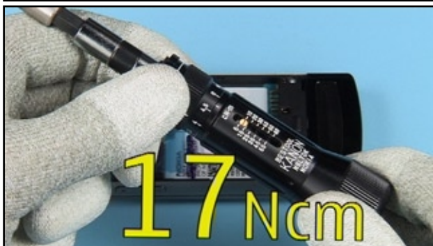
55. Set the correct torque.
