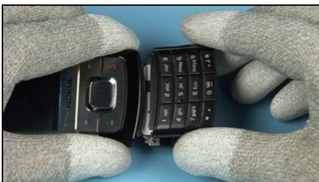
21. If both clips are released properly, the BOTTOM KEYMAT can be lifted up.
