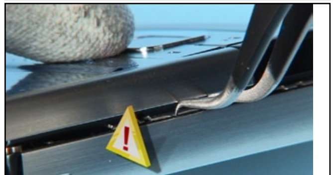
8. Now swing up the tweezers in order to lever out the metal latches.
