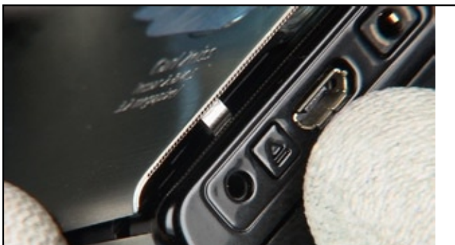
3. Unlock and remove the BATTERY COVER.
