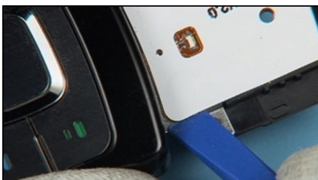
27. Carefully lever up the edges of the BOTTOM FLEX...
