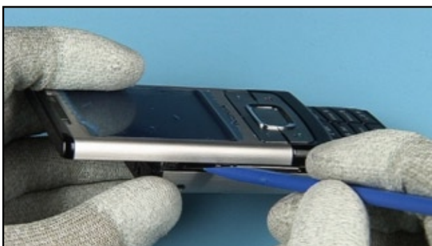
13. Insert the SS-93 at the shown position.
