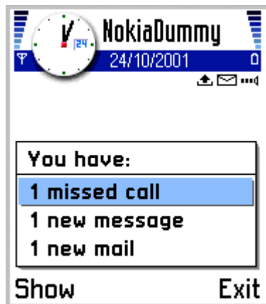
Figure 5-43: A grouped soft notification. The height of the window is dynamic and depends on the number of lines in the list.
