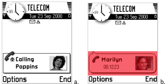
Figure 6-6. Phone application examples: a. Creating an outgoing call; b. Active call going on.
