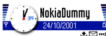
Figure 5-52. Signal and battery indicators on the sides of the status pane. Other status indicators are visible below the navi pane.
