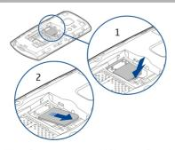
Press the release spring (1), and slide out the SIM card (2).
