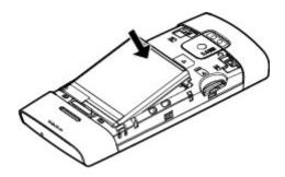
4 To replace the back cover, direct the top locking catches toward their slots, and press down until the cover locks into place.
