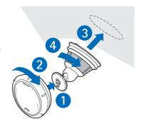
If the ambient temperature is below +15°C (60°F), carefully warm the surface and the suction cup with a hair dryer to ensure a firm grip on the windscreen. Ensure that you do not heat the windscreen excessively to avoid damage to it.
