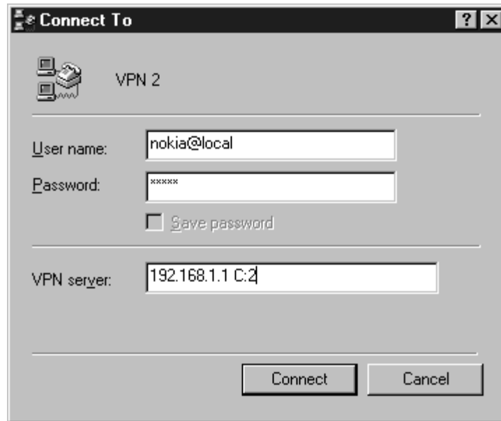
Figure 2-5 Choosing the VCC2 for tunneling example
