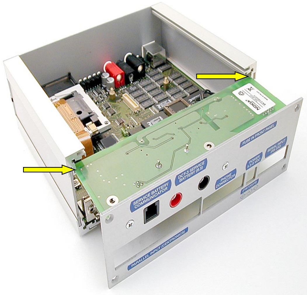
Pic 26 DCT3 power supply module (ACS-10) installation 1
