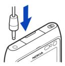
Do not connect products that create an output signal, as this may damage the device. Do not connect any voltage source to the Nokia AV connector. If you connect an external
