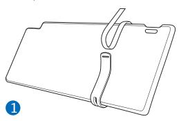
Thread the strap through the slot on the clip. Tighten the strap to keep the speakerphone securely in place, and firmly press the hook and loop end of the strap against the felt on the strap (2).
