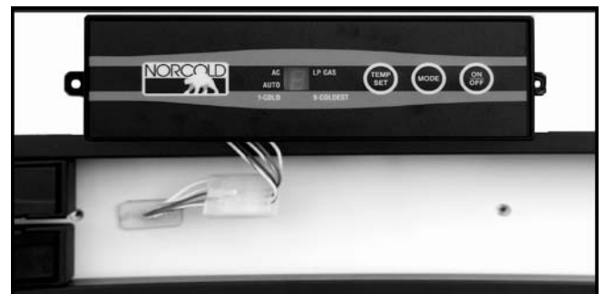
Figure 41. Wire Harness Connection.
