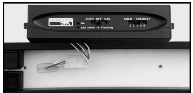
Figure 38. Wire Harness Connection.
