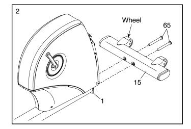
3. Orient the Upright (2) as shown. Have a second person hold the Upright near the front of the Frame (1).
