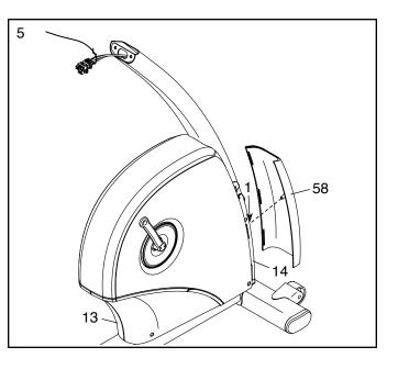
6. Orient the Upright Cover (57) as shown. Hold the Upright Cover near the Upright (2), and insert the wires upward through the Upright Cover.
