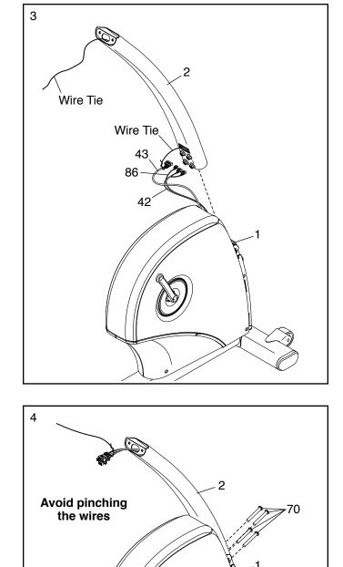
4. **Tip: Avoid pinching the wires.** Slide the Upright (2) onto the Frame (1).
