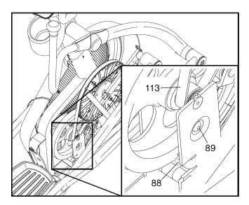
Reattach the right disc by pressing it firmly into the right disc mount.
