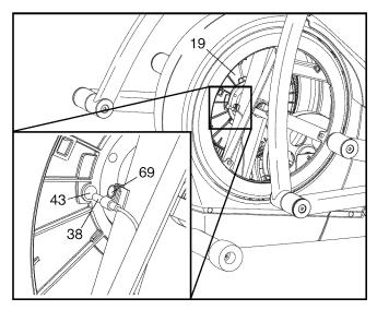
Reattach the left disc by pressing it firmly into the left disc mount.
