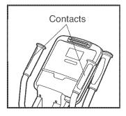
sure your heart rate, hold the handgrip pulse sensor with your palms resting against the metal contacts. Avoid moving your hands or gripping the contacts tightly.
