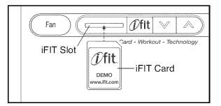
Next, select the desired program on the iFIT Card by pressing the increase and decrease buttons next to the iFIT slot.
