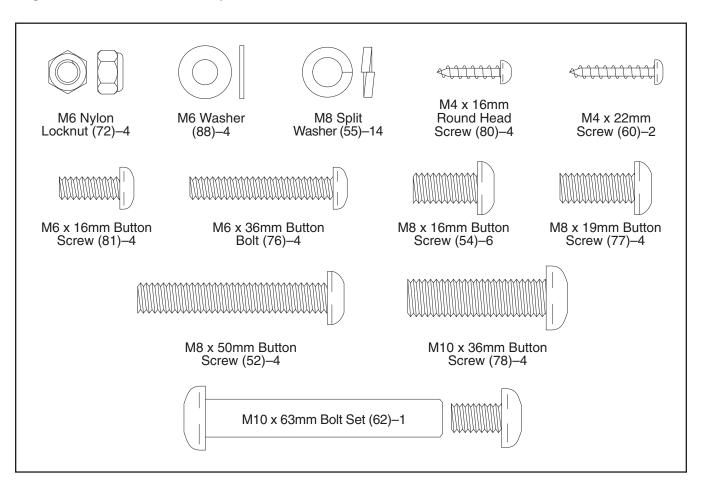
Attach the Left Front Stabilizer (15) to the left side of the Frame (1) with three M8 x 16mm Button Screws (54) and three M8 Split Washers (55).
