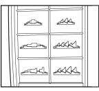
When a preset program is selected, a profile of the resistance settings of the program will scroll across the matrix and the maximum resistance setting of the program will flash in the lower display. A few seconds after a program is selected, the upper display will show how long the program will last.
