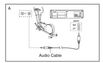
B. Plug one end of a long 1/8" to RCA stereo audio cable (available at electronics stores) into either jack on the console. Plug the other end of the cable into an RCA Y-adapter (available at electronics stores). Next, remove the wire that is currently plugged into the AUDIO OUT jack on your VCR and plug the wire into the unused side of the Yadapter. Plug the Y-adapter into the AUDIO OUT jack on your VCR.
