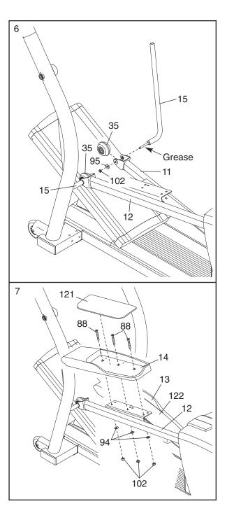
8. Apply a thin film of the included high-temperature lubricant to both Pivot Shafts (15).
