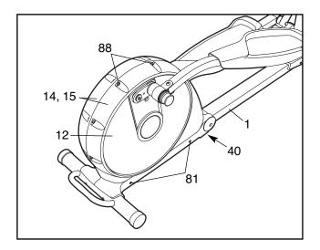
Adjust the position of the Side Shields (14, 15) until the Discs (12) no longer rub against them, and then tighten the Bolt Sets (88) and the M4 x 19mm Screws (81).
