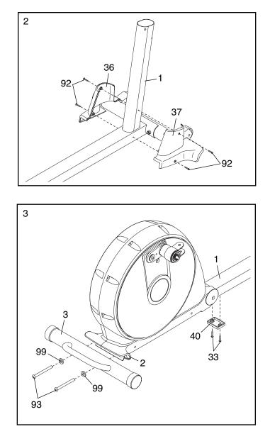
With the help of another person, carefully tip the elliptical exerciser onto its side. Attach the Center Foot (40) to the Frame (1) with two M4 x 16mm Blunt Screws (33). Then, return the elliptical exerciser to the upright position.
