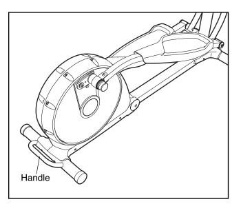
To unfold the elliptical exerciser, hold the handle, press the latch button, and then lower the frame to the floor.
