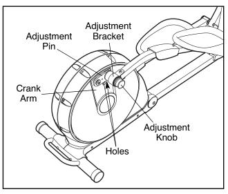
Adjust the other side of the elliptical exerciser in the same way; make sure that each side of the elliptical exerciser is adjusted to the same stride length.
