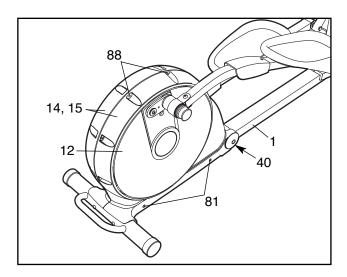
Adjust the position of the Side Shields (14, 15) until the Discs (12) no longer rub against them, and then tighten the M8 x 25mm Bolt Sets (88) and the #8 x 1/2" Screws (81).
