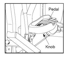
the pedals forward or backward to the desired position, and then retighten the knobs. Make sure that both pedals are in the same position.
