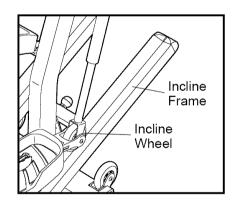
frame where the incline wheels make contact with it. Other parts of the elliptical crosstrainer can also be cleaned in this way. **Never use abrasives or solvents.**
