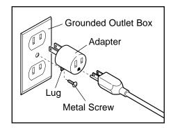
available. The temporary adapter should be used only until a properly grounded outlet can be installed by a qualified electrician.
