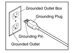
current to reduce the risk of electric shock. This product is equipped with a cord having an equipmentgrounding conductor and a grounding plug. Plug the power cord into an appropriate outlet that is properly installed and grounded in accordance with all local codes and ordinances. This product is for use on a nominal 120-volt circuit. Important: The elliptical crosstrainer is not compatible with GFCI-equipped outlets.
