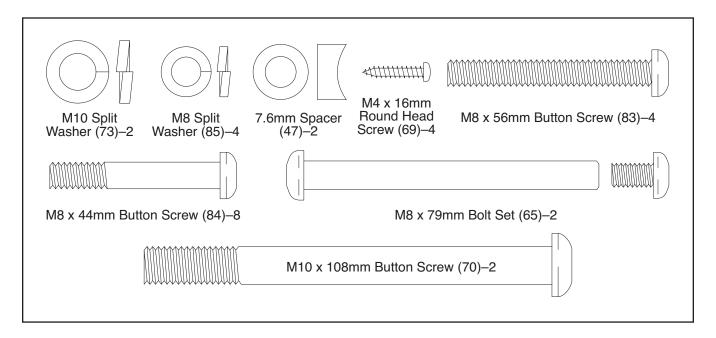
Identify the Front Stabilizer (8). While another person lifts the front of the Frame (1) and holds the Pedal Legs (4, 5) in the position shown, attach the Front Stabilizer to the Frame with four M8 x 44mm Button Screws (84) and a Support Plate (64).
