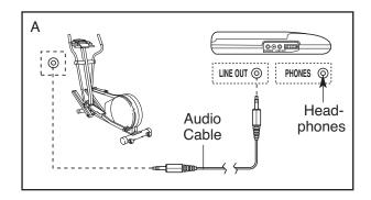
B. Plug one end of the audio cable into the jack beneath the console. Plug the other end of the cable into a 1/8" Y-adapter (available at electronics stores). Plug the Y-adapter into the PHONES jack on your CD player. Plug your headphones into the other side of the Y-adapter.
