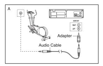
B. Plug one end of the audio cable into the jack beneath the console. Plug the other end of the cable into the adapter. Plug the adapter into an RCA Y-adapter (available at electronics stores). Next, remove the wire that is currently plugged into the AUDIO OUT jack on your VCR and plug the wire into the unused side of the Y-adapter. Plug the Y-adapter into the AUDIO OUT jack on your VCR.
