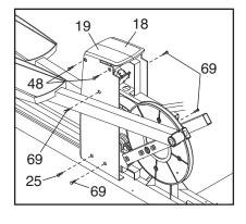
removed from; the Screws will later need to be reattached in the same holes. Carefully separate and remove the Flywheel Covers.
