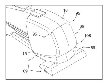
Next, the Right and Left **Flywheel Covers** (18, 19) must be removed. Remove the indicated Screws (69, 108) from the Flywheel Covers. Note which hole each Screw is
