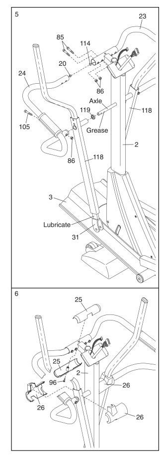
Apply a liberal amount of grease to the barrel of each M8 x 79mm Bolt Set (65).
