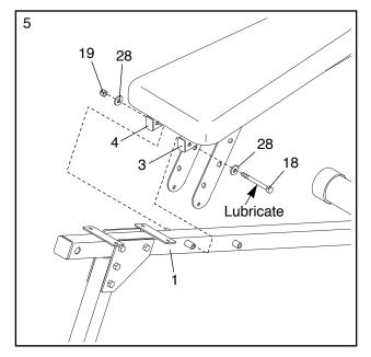
6. Note that the brackets on the Backrest Frames (3, 4) have three sets of oval adjustment holes and one set of round holes.
