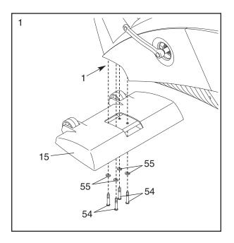
While another person lifts the rear of the Frame (1), attach the Rear Stabilizer (16) to the Frame with four M8 x 40mm Button Screws (54) and four M8 Split Washers (55).
