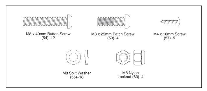
Identify the Front Stabilizer (15). While another person lifts the front of the Frame (1), attach the Front Stabilizer to the Frame with four M8 x 40mm Button Screws (54) and four M8 Split Washers (55).
