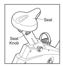
loosen it. Slide the seat forward or backward to the desired position, and then firmly tighten the seat knob.
