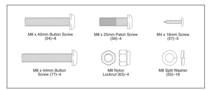
Identify the Front Stabilizer (15). While another person lifts the front of the Frame (1), attach the Front Stabilizer to the Frame with four M8 x 40mm Button Screws (54) and four M8 Split Washers (55).
