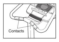
measure your heart rate, hold the handgrip pulse sensor with your palms resting on the contacts. **Avoid moving your hands.**  When your pulse is detected, the Heart Rate indicator above the right display will begin to flash, one or two dashes (--) will
