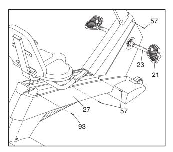
Locate the Reed Switch (46). Turn the Right Crank Arm (23) until the Magnet (30) is aligned with the Reed Switch. Loosen, but do not remove, the indicated M4 x 16mm Screw (57). Slide the Reed Switch slightly closer to or away from the Magnet. Then, retighten the Screw. Turn the Right Crank Arm for a moment. Repeat until the console displays correct feedback. When the Reed Switch is correctly adjusted, reattach the right side shield and the right pedal.
