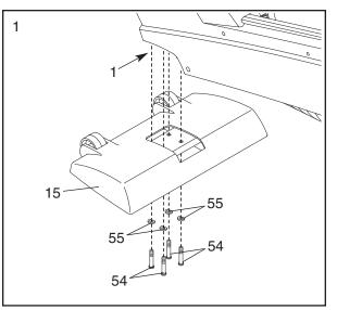
2. While another person lifts the rear of the Frame (1), attach the Rear Stabilizer (16) to the Frame with four M8 x 40mm Button Screws (54) and four M8 Split Washers (55).
