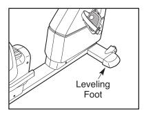
rocks slightly during use, turn one or both of the leveling feet under the front stabilizers until the rocking motion is eliminated.
