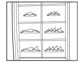
When a preset program is selected, a profile of the resistance settings of the program will scroll across the matrix and the maximum resistance setting of the program will flash in the lower display. A few seconds after a program is selected, the upper display will show how long the program will last.
