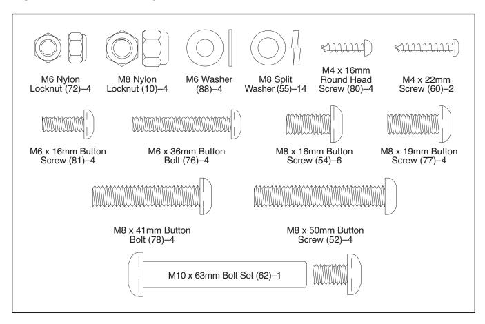
1. Attach the Left Front Stabilizer (15) to the left side of the Frame (1) with three M8 x 16mm Button Screws (54) and three M8 Split Washers (55).
