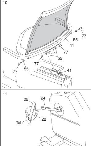
11. Identify the Left Pedal (22), which is marked with an "L." Using an adjustable wrench, firmly tighten the Left Pedal counterclockwise into the Left Crank Arm (24). Tighten the Right Pedal (not shown) clockwise into the Right Crank Arm (not shown). Important: Tighten both Pedals as firmly as possible. After using the exercise cycle for one week, retighten the Pedals.
