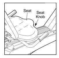
seat knob snaps into one of the holes in the seat rail.
