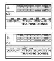
*right* of the lit indicators is flashing (see drawing a), increase your pace. If an indicator to the *left* of any lit indicator is flashing (see drawing b), decrease your pace. When no indicator is flashing, your heart rate is near the current heart rate setting. **Important: The heart rate settings are intended only to provide motivation. Your actual heart rate may be slower than the current heart rate setting. Make sure to exercise at a pace that is comfortable for you.**
