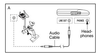
B. Plug one end of the audio cable into the jack beneath the console. Plug the other end of the cable into a 3.5 mm (1/8 in.) Y-adapter (available at electronics stores). Plug the Y-adapter into the PHONES jack on your CD player. Plug your headphones into the other side of the Y-adapter.
