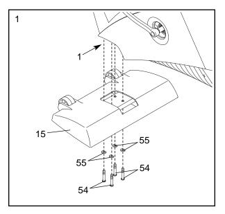
While another person lifts the rear of the Frame (1), attach the Rear Stabilizer (16) to the Frame with four M8 x 40mm Button Screws (54) and four M8 Split Washers (55).
