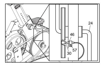
Turn the Right Crank Arm (23) for a moment. Repeat until the console displays correct feedback. When the Reed Switch (46) is correctly adjusted, reattach the Right Side Shield (27) and the Right Pedal (21).
